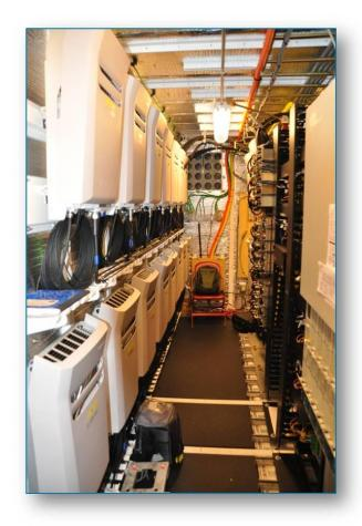
Distributed antenna systems increase both the coverage and capacity of cellular networks, but they typically are planned and deployed over several months. The development of a portable DAS system "allows us to deploy a very, very robust network in days if not hours," says Doublin. Clearly, the technology has major implications for public safety systems and first responders.
